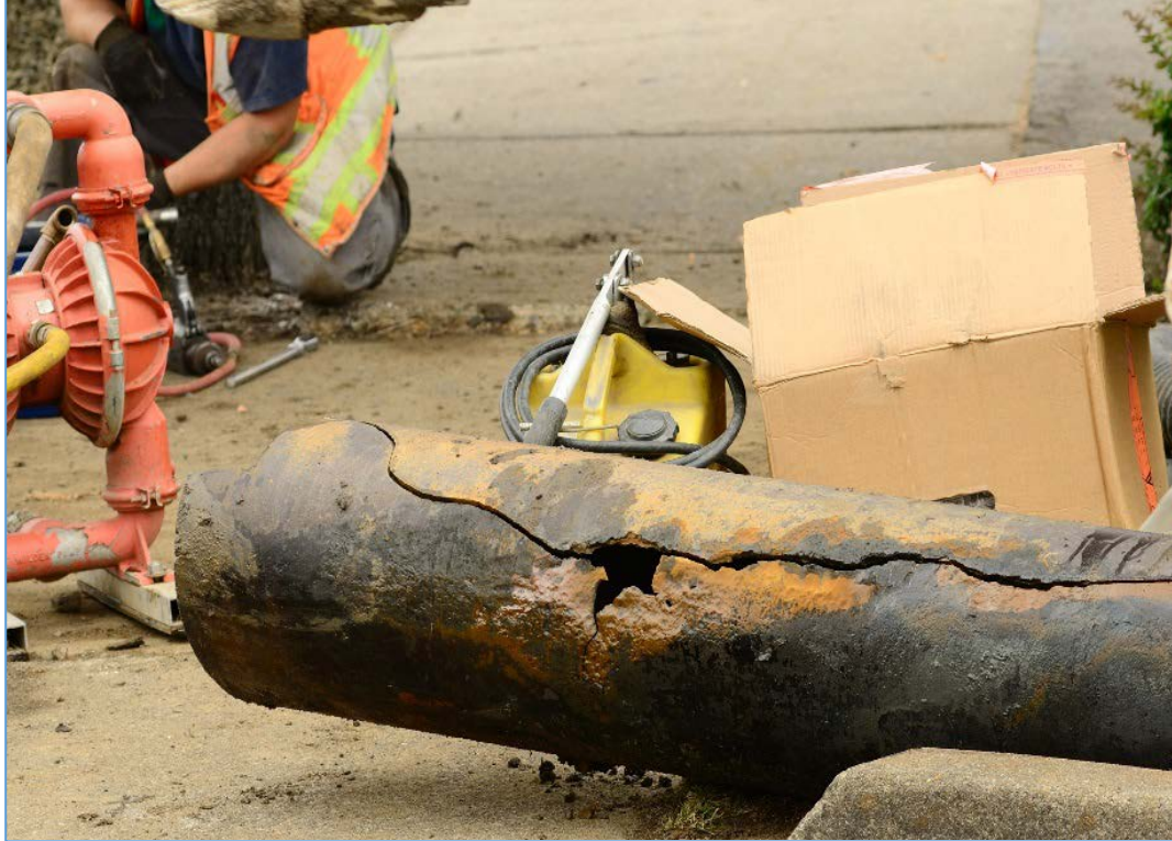
Figure 3: Steam Distribution – Water Hammer
